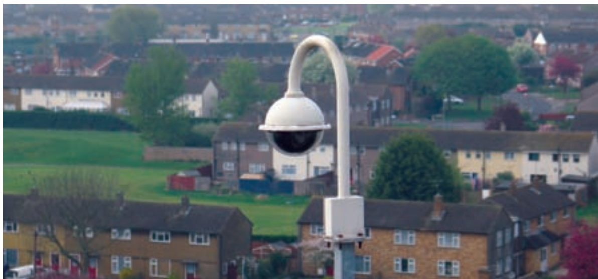
Camera over Swindon rooftops, by 802 Global. To tap into a wireless IP CCTV signal would require an antenna in the line of sight.
